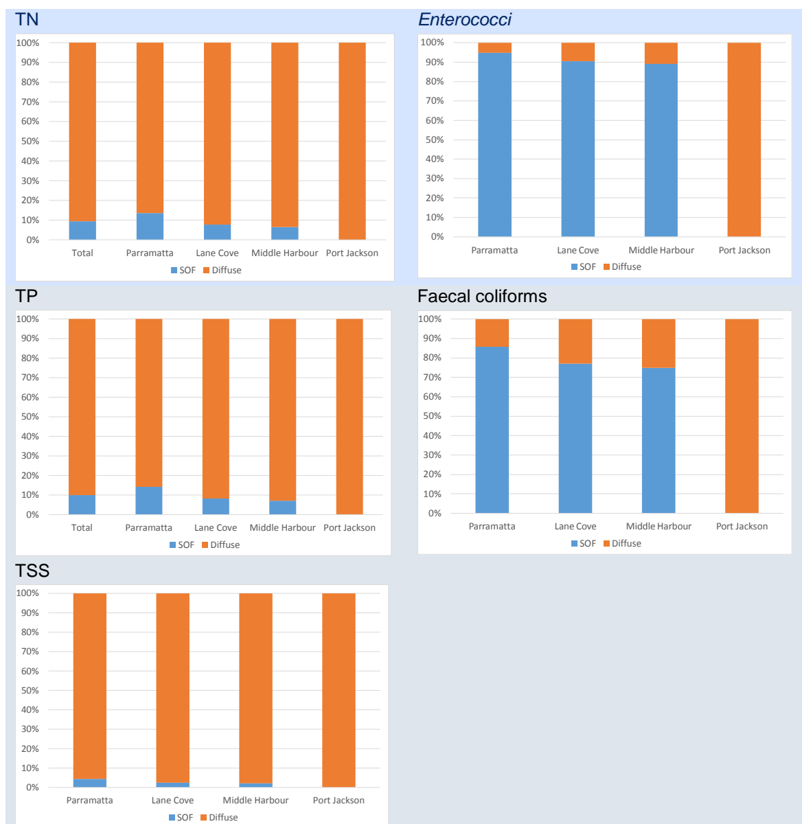
Figure 3.3 The proportion of pollutants that is contributed from sewer overflows (sof) versus diffuse sources for the four major subcatchments in the Sydney Harbour catchment (sof data provided by Sydney Water for Port Jackson was incomplete).
